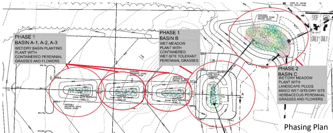
Naturalizing basins involves placing native species into existing basin bottom and the surrounding sloped edges. This Best Management Practice (BMP) helps improve water quality, enhance groundwater recharge, and reduce stormwater volumes that discharge to Fox Hollow lake and other local waterways. Students were setting the riverstone rocks aside, planting into the soil, and crowned each plant with topsoil. This secured the plants with nutrients and the chance for better root growth.
